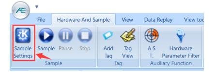
4) In the "Sample settings" >> "Hit Feature", click "Refresh" button at the bottom right corner of the window. After refreshing the hardware, it shows how many channels it recognizes at the bottom. Make sure to tick at least one of the channels that the EX PARA BOX connects with (should #1-4).
