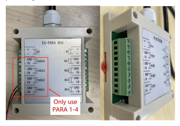
2) Insert the EX\_PARA Box into the acquisition card's External card socket of the U3H chassis. The AE acquisition card with the EX\_PARA BOX must be the first AE card in the chassis and the chassis "NUM" must be "00". It should have been all setup well before delivery. Double check these hardware setups just in case it might be accidentally bumped during delivery or unpacking.
